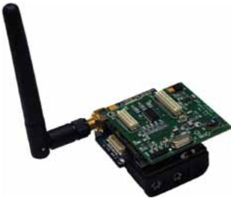
Figure 2: Imote2/ISM400 wireless smart sensor node.
