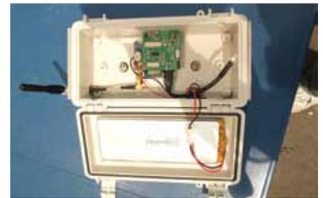
Figure 4: Example of wireless smart sensor nodes deployed on the Jindo Bridge.
